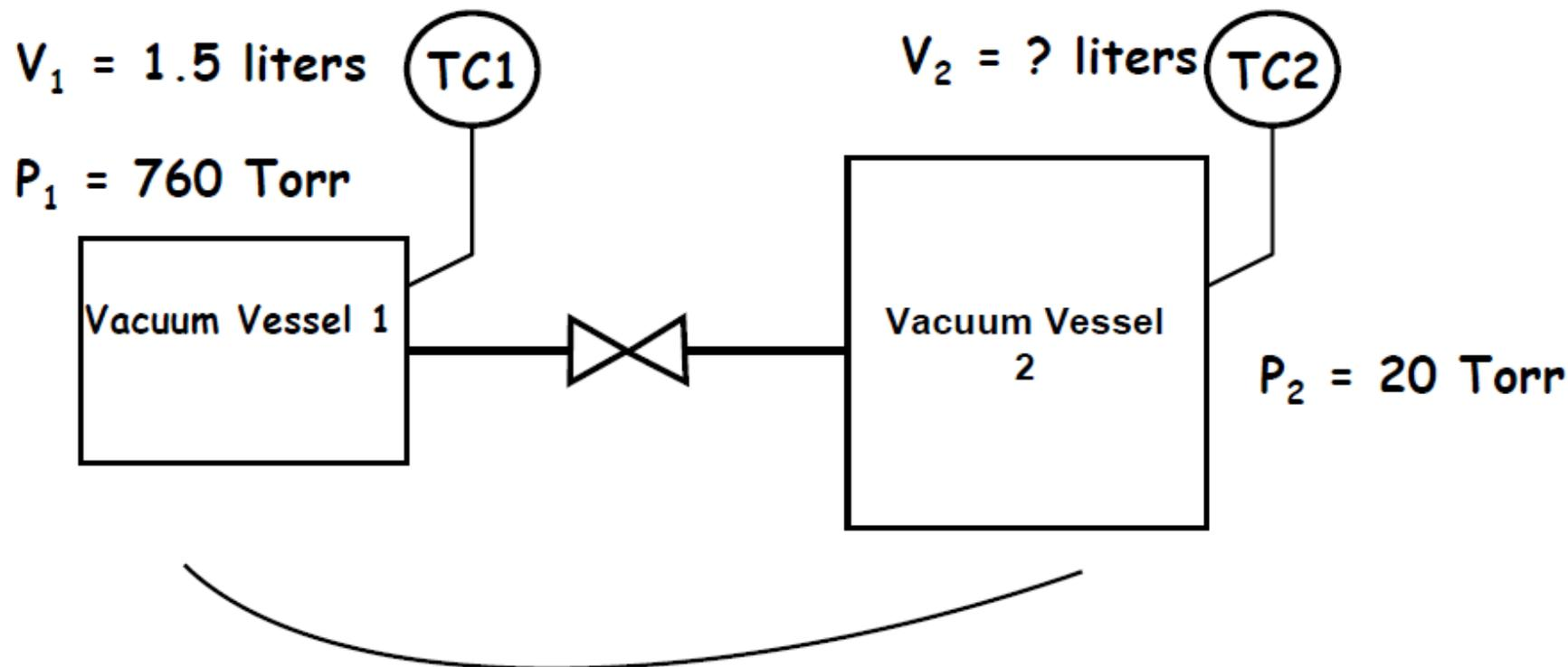
*Boyle's Law can also be used to expand gauge calibration range via expansion*
