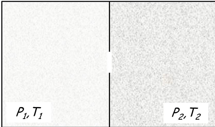
At molecular flow ( $\lambda \gg d$ ), gas flux through an orifice:
