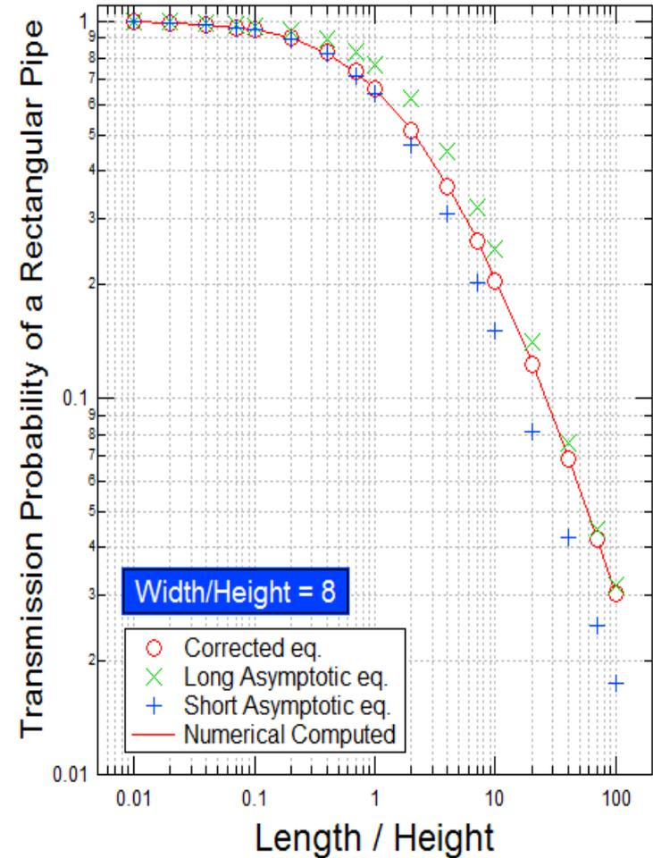
*Comparing numerically computed transmission with  $\alpha_s$ ,  $\alpha_l$  and corrected  $\alpha$ .*
