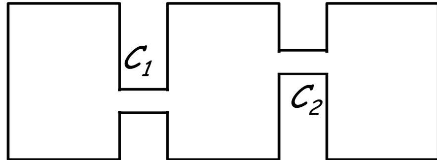
*The series elements must be separated by large volumes, so that the molecular flow is re-randomized before entering next element*
